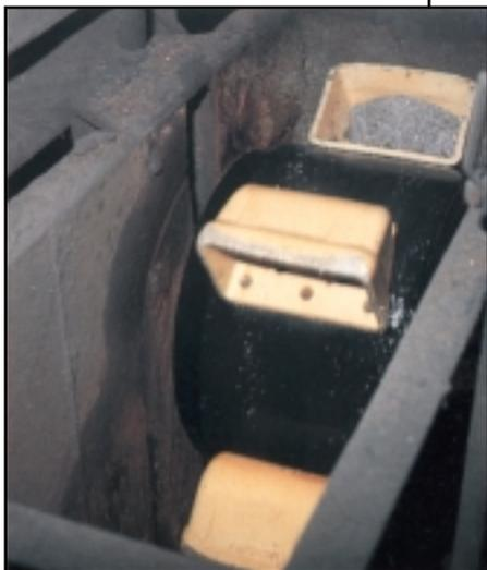
**Maxi-Tuff® buckets deliver hot, wet steel shot to drying hoppers.**
