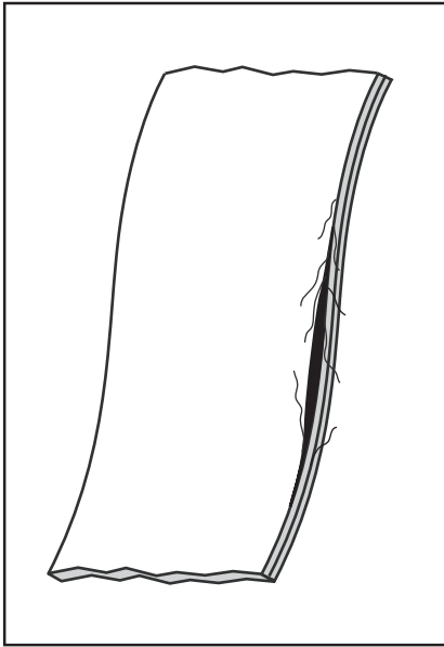
FRAYS - Indicate belt is off track and running to one side
