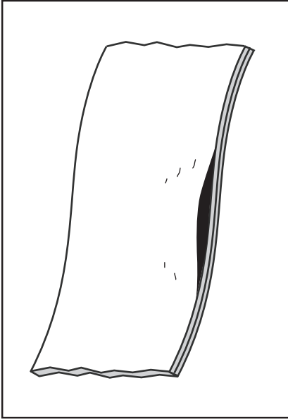
EDGE DELAMINATION - Delamination of belt or exposed fabric
