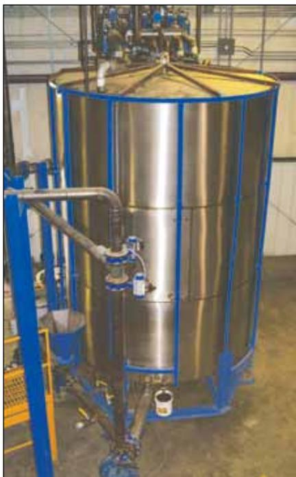
*Liquid feeds are mixed in this 6,000-gallon tank from Southern Metal Fabricators.*
