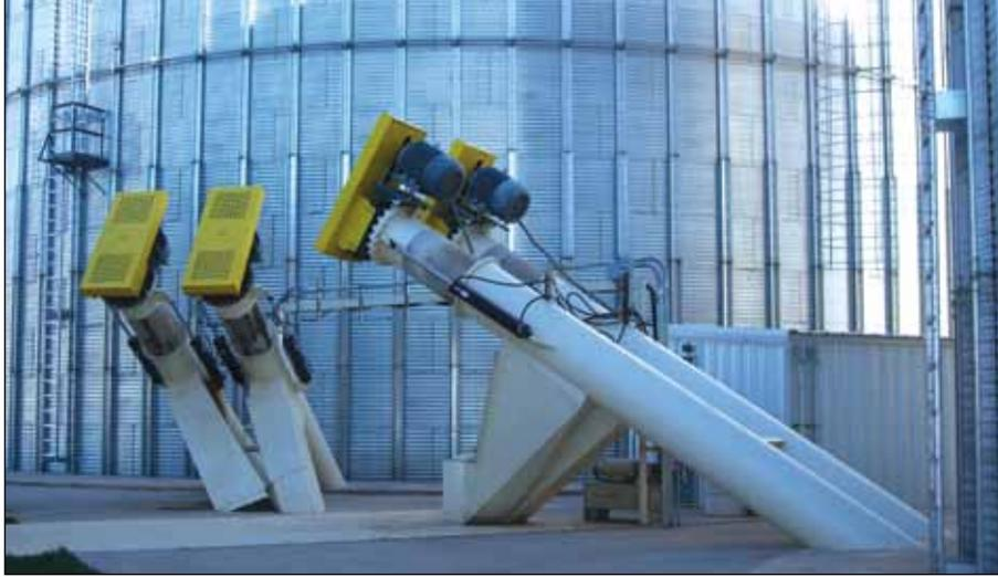
*A pair of Pitcock telescoping augers per tank empty the two Behlen steel tanks, which have 40-degree concrete hopper floors.*
