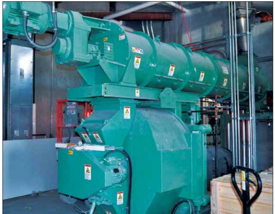
One of two CPM Model 7936-14 pellet mills capable of producing 50 tph.
