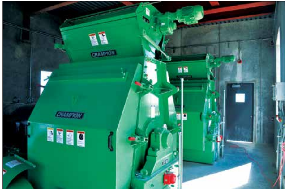
Pair of CPM Roskamp Champion hammermills for grinding incoming corn in the new tower.
