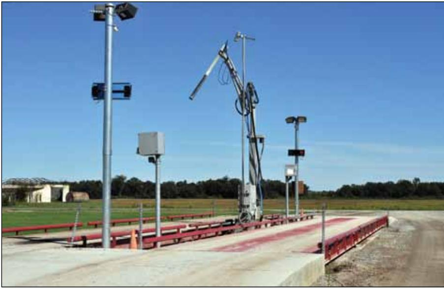
*Twin 80-foot Rice Lake pitless truck scales weigh inbound and outbound trucks. Intersystems provided the truck probe, and CompuWeigh provided the scale automation system.*
