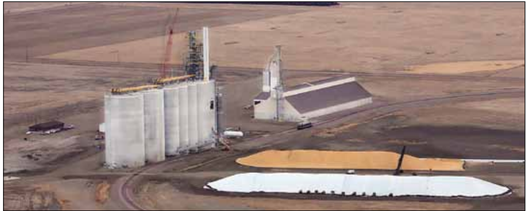
Aerial view of Gavilon's new rail terminal near Kimball, SD including a 2.2-million-bushel elevator, 4 million bushels of outdoor temporary storage, 41,590-ton fertilizer plant, and 10,000-foot loop track. Aerial photo by JH Photography, Spencer, IA.
