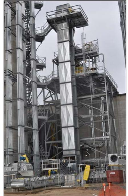
*InterSystems 60,000-bph shipping leg deposits grain onto an overhead 60,000-bph covered belt conveyor out to the river.*
