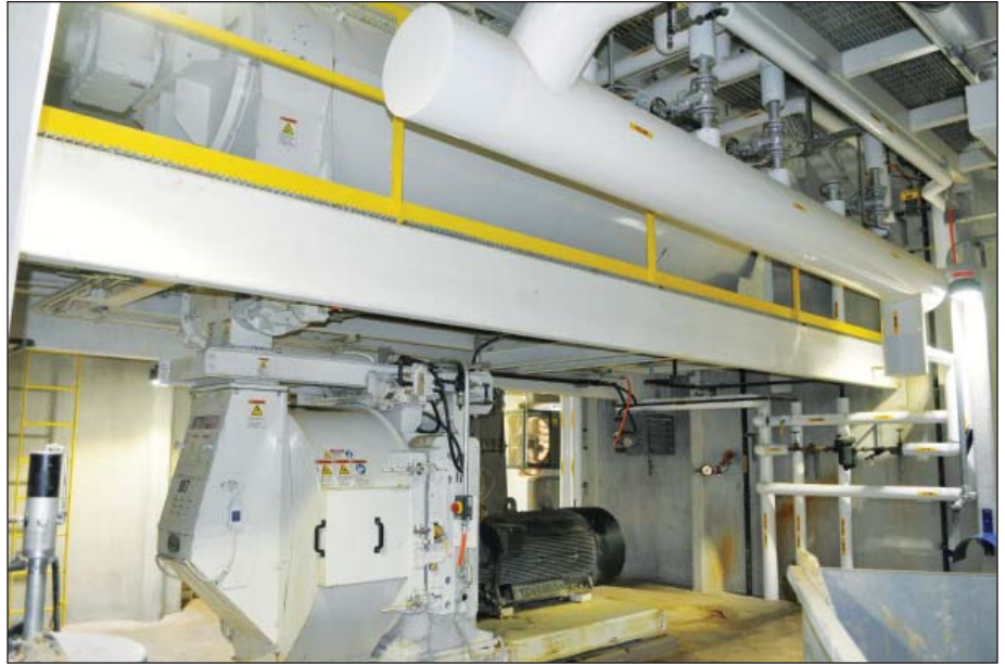
Combination steam conditioner and hygieniser ensure sterile feed going into the pellet mill below. All equipment is from CPM.
