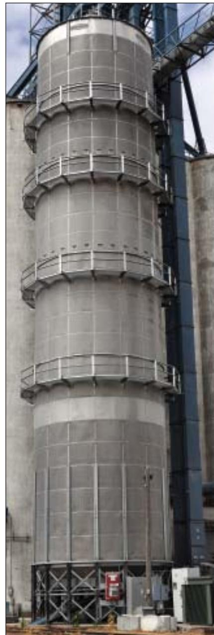
Relatively new 7,000-bph Brock natural-gas-fired grain dryer was built as part of the steel annex project.
