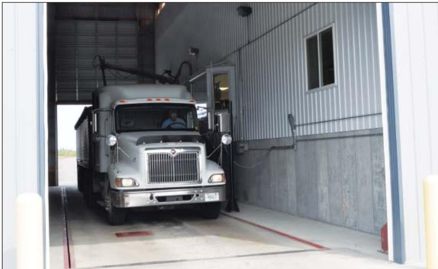
*An incoming grain truck is weighed and probed in an enclosed scalehouse bay.*
