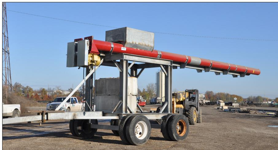
Portable auger system has been loading grain from the facility bulkweigher directly into 40-foot shipping containers.
