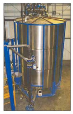
Liquid feeds are mixed in this 6,000-gallon tank from Southern Metal Fabricators.
