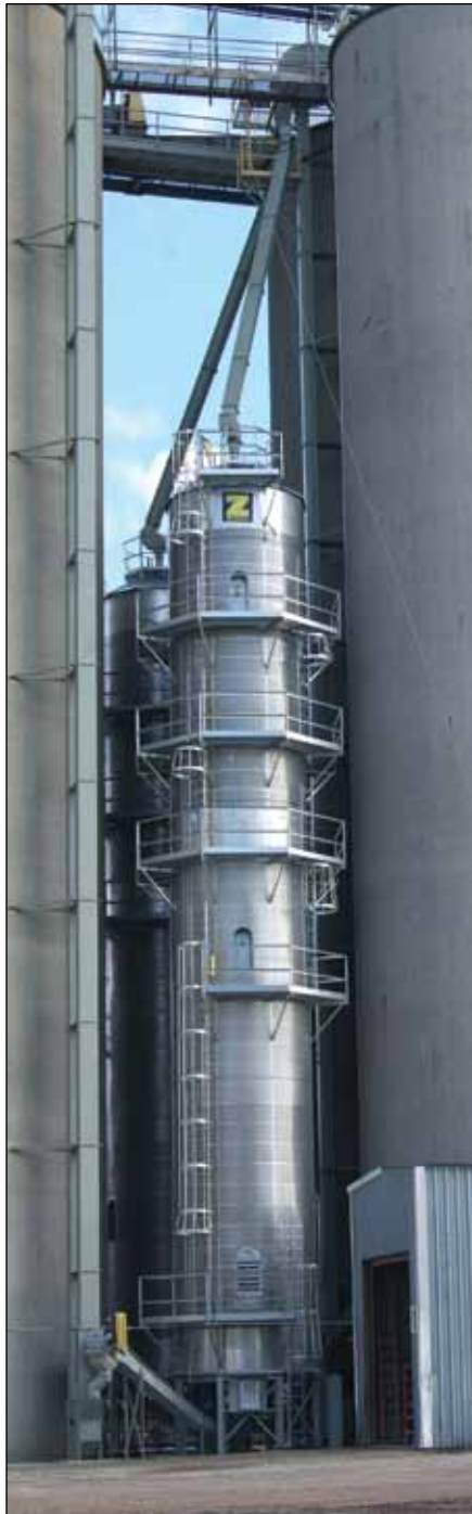
Two new 2,500-bph Zimmerman tower dryers, selected instead of a single 5,000-bph model for space reasons.
