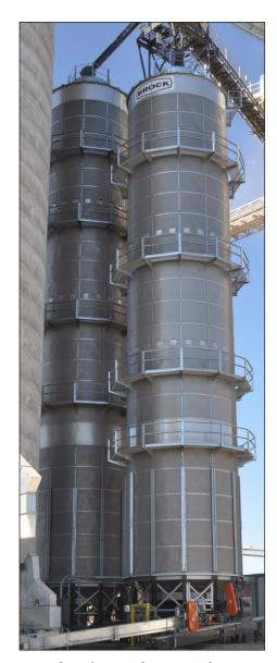
Pair of Brock tower dryers provide 8,700 bph of drying capacity at five points of moisture removal.
