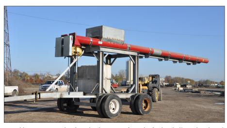
Portable auger system has been loading grain from the facility bulkweigher directly into 40-foot shipping containers.
