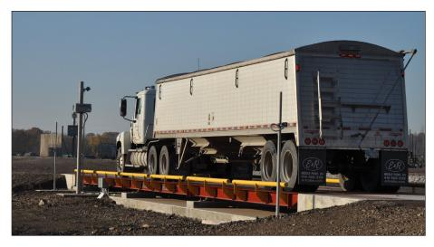
Inbound truck is weighed on a 72-foot Brechbuhler scale while the driver awaits instructions via a CompuWeigh SmartView digital message board. Ground-level photos by Ed Zdrojewski.
