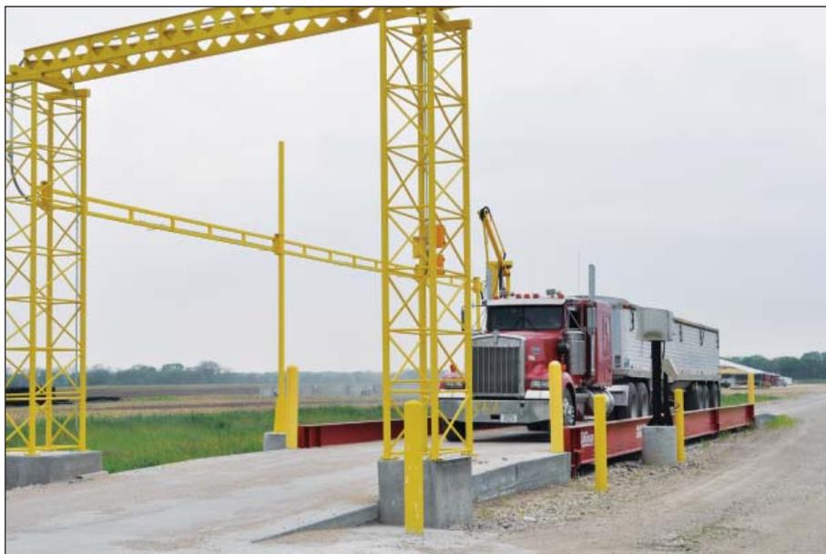
Trucker pulls onto a Rice Lake outbound scale, which is outfitted with Comco scale automation and a Gamet truck probe.
