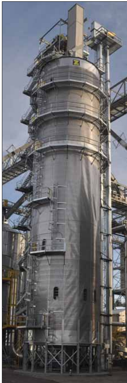
Propane-fired Zimmerman tower dryer is rated to dry 7,500 bph at five points of moisture removal.
