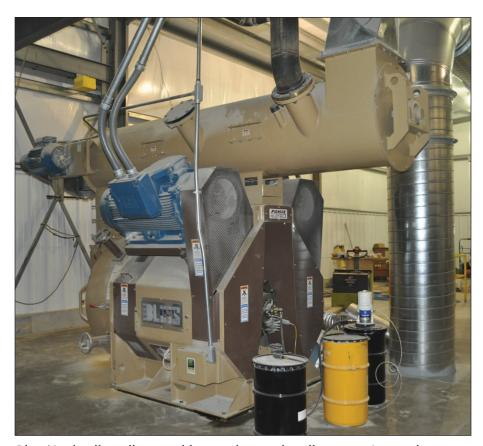
Bliss 45-tph pellet mill is topped by a conditioner that allows up to 51 seconds retention time for incoming mash feed.
