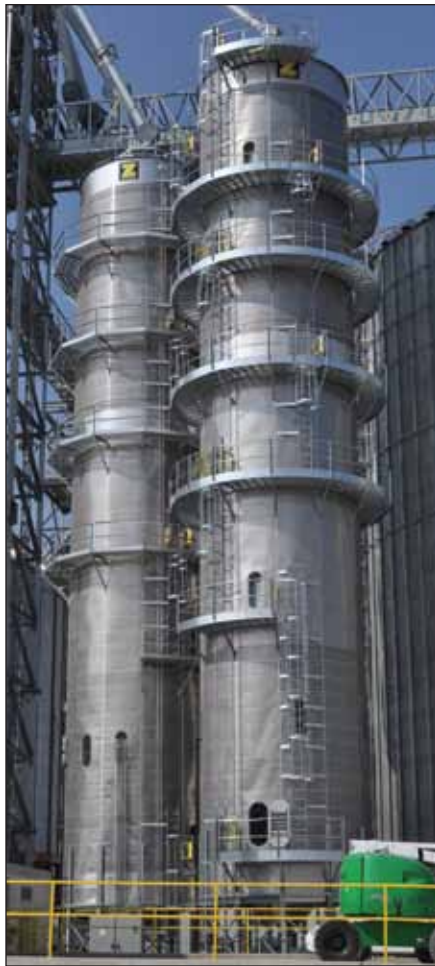
Twin 4,700-bph Zimmerman tower dryers allow for increased flexibility during high or low volumes. Ground-level photos by Ed Zdrojewski.
