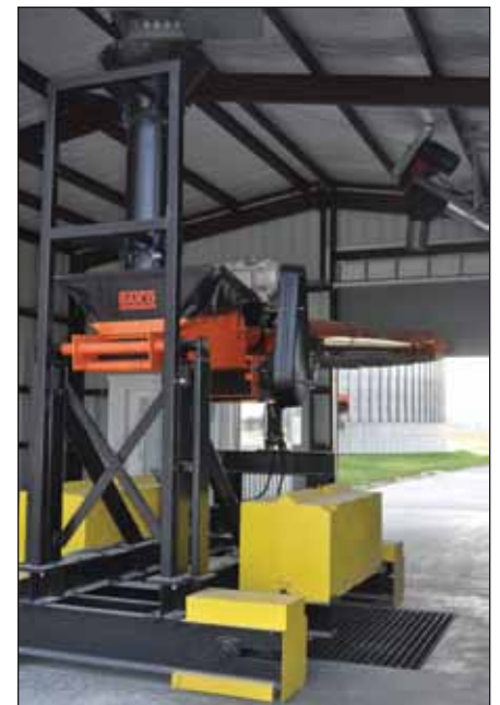
Batco belt loader for loading 20-foot containers destined for a rail container yard 25 miles away.
