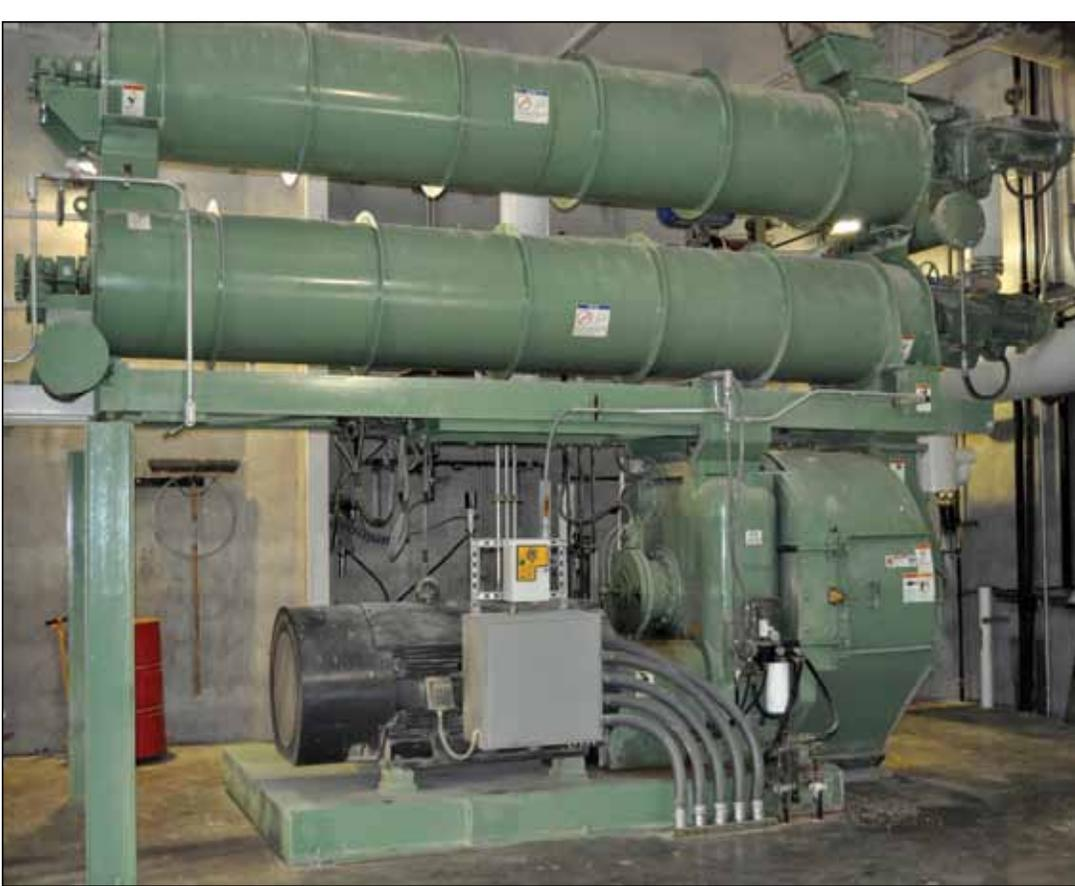
*The plant's CPM pellet mill with double-stack steam conditioner, generally operating at 85 tph.*
