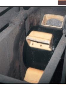
Maxi-Tuff<sup>a</sup> buckets deliver hot, wet steel shot to drying hoppers.
