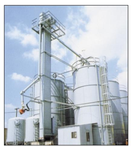
Halliburton's 60-foot tall bucket elevator elevates sand, which empties into a piping system leading to storage tanks or to trucks that haul the sand to oil fields the company services.
