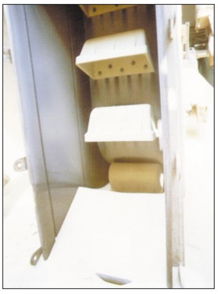
As the elevator buckets make a 180 degree turn at the elevator's bottom, they fill with sand to be carried up to a downspout for discharge.
