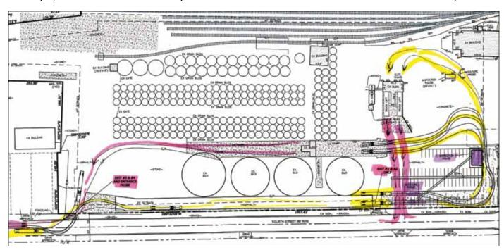
Schematic of the Blanchard Valley grain complex in Fostoria. The yellow lines show the route of trucks through the facility prior to the start of the newest construction in 2010, while the purple lines show the rerouting that removed a lot of truck traffic that used to stand along Fourth Street waiting to dump. Illustration courtesy of Blanchard Valley Farmers Cooperative.
