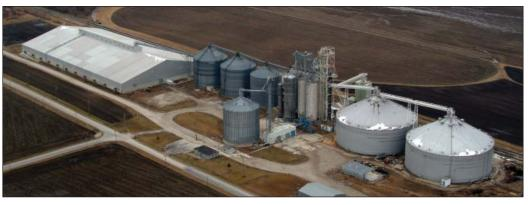
Prairie Central's rail terminal north of Pontiac, IL. New 10,000-bph Zimmerman dryer is visible near the center of the photo.
