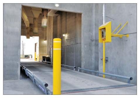
Loadout bay and METTLER TOLEDO truck scale are designed to load up to 60 feed trucks per day.
