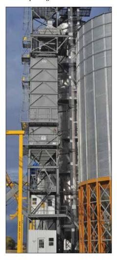
The terminal's 80,000-bph bulk weigh loadout scale from C&A Scales is topped by an Intersystems gravity screener.
