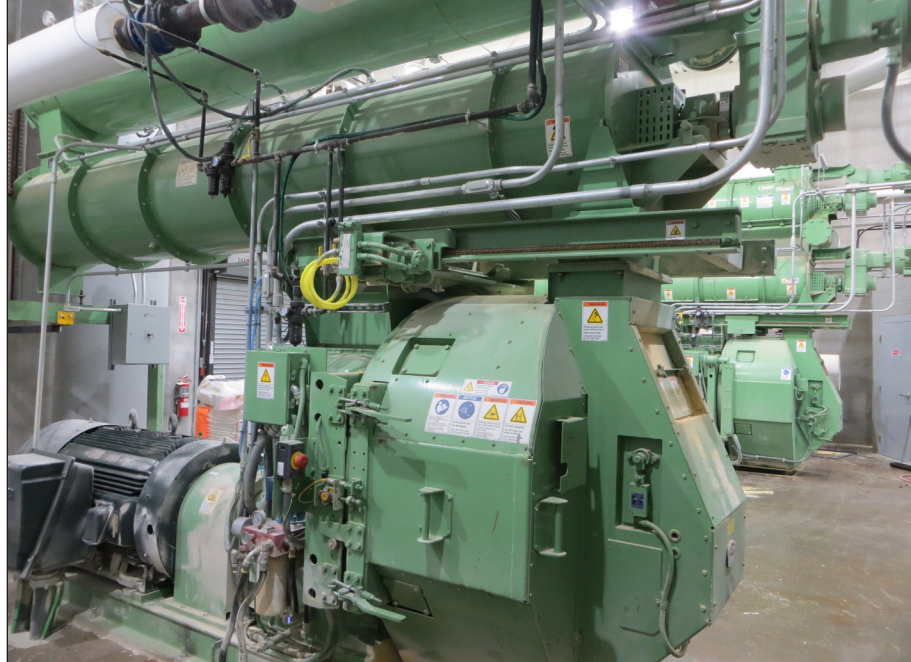
ABOVE: Two 70-tph CPM Roskamp Champion pellet mills with steam conditioners. BELOW: Two Bliss counterflow pellet coolers operate at approximately 75 tph.
