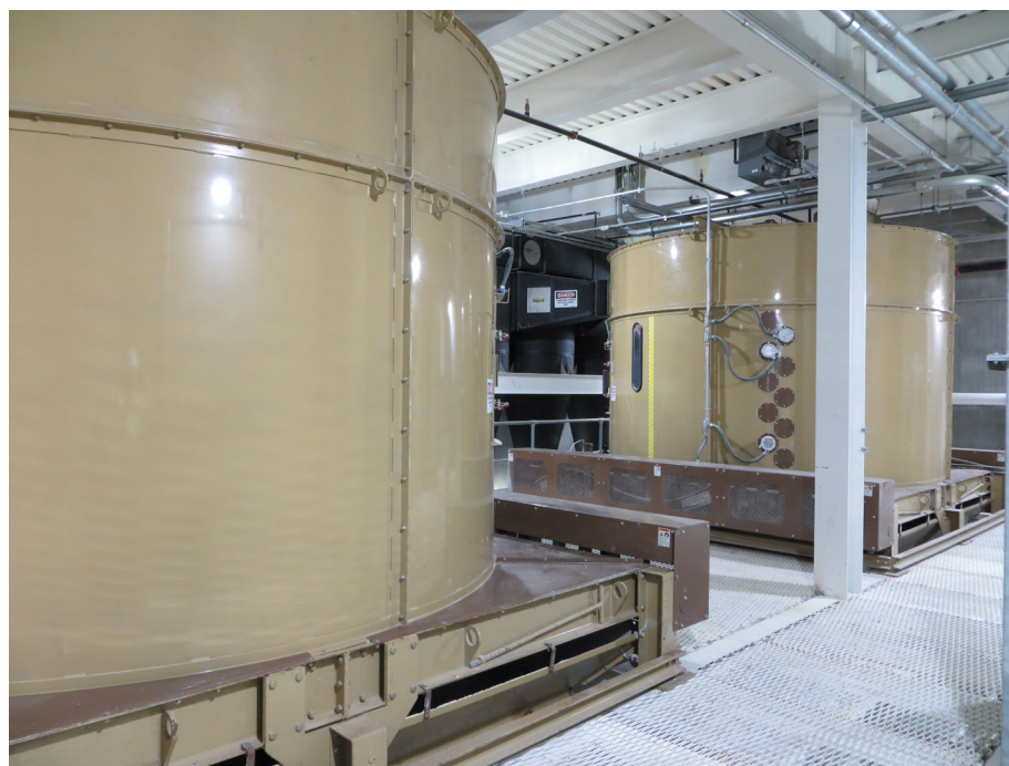
ABOVE: Two 70-tph CPM Roskamp Champion pellet mills with steam conditioners. BELOW: Two Bliss counterflow pellet coolers operate at approximately 75 tph.
