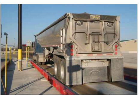
Outbound truck is weighed on a new Rice Lake platform scale, while driver takes his scale ticket from a printer that is part of a CompuWeigh SmartTruck scale management system.
