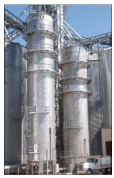
Two Zimmerman tower dryers installed in 2006, the left dryer rated at 4,700 bph and the other at 4,000 bph at five points of moisture removal.
