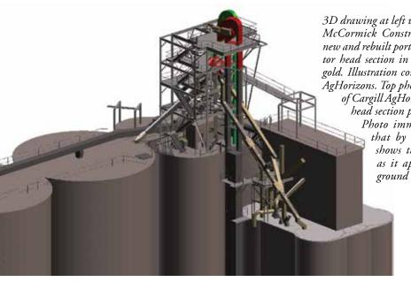
3D drawing at left was developed by McCormick Construction showing new and rebuilt portions of the elevator head section in red, green, and gold. Illustration courtesy of Cargill AgHorizons. Top photo, also courtesy of Cargill AgHorizons, shows the head section prior to upgrade. Photo immediately below that by Ed Zdrojewski shows the head section as it appears from the ground today.
